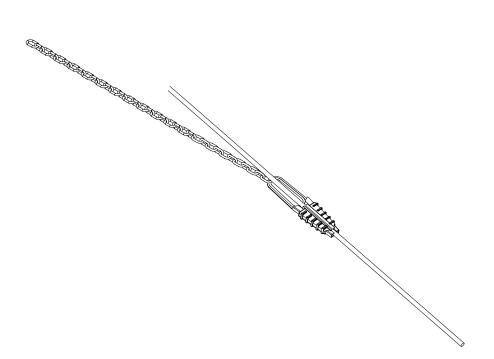
Secure the cable on the hook. Then lower the sensor until it is fully submersed in the water.
