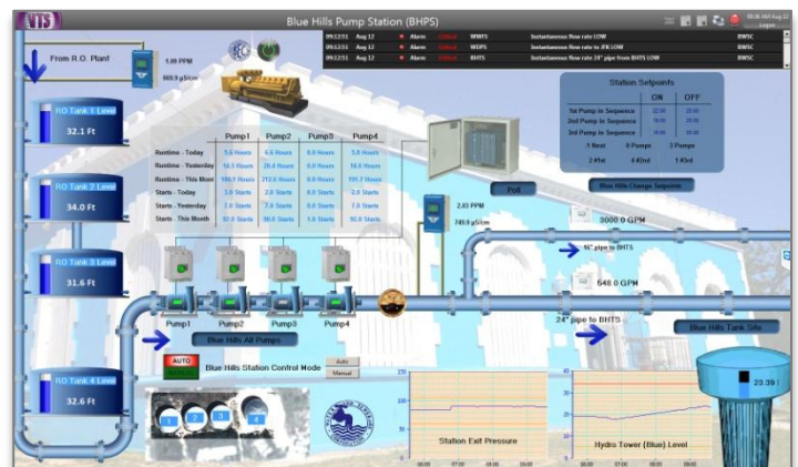
SCADA Pump Monitor & Control – Blue Hills Station Overview
