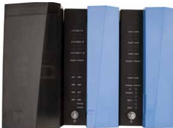
ACE1000 Remote Terminal Unit with covers
